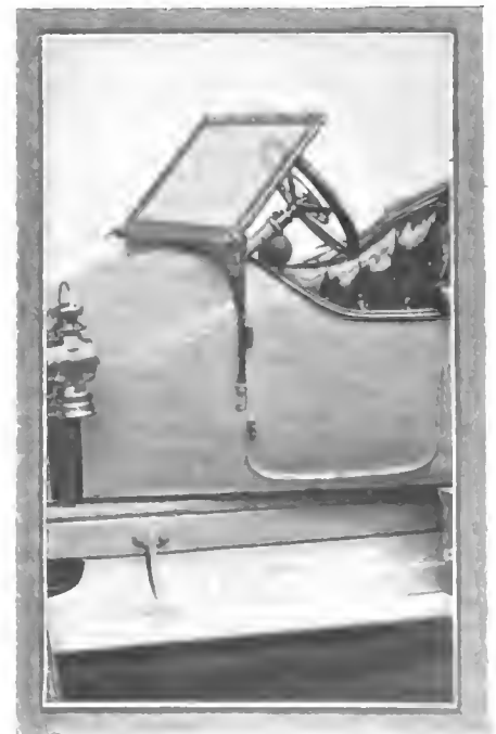
Fig. 12—Method of fitting a top to a curved cowl. The shield is fitted with a locking device whereby the position can be altered at will
